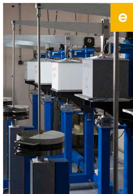
The long-term deformation of an insulation material can influence its performance. Creep testing is designed to categorize the characteristics of the product relative to the requirements imposed by installation rules.
