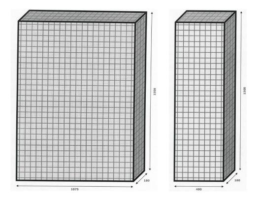
The support, defined in standard EN 13823, is placed at the back of the cages.
