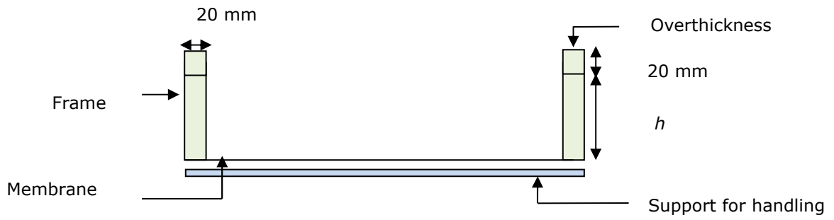
Figure 1 - Example of frame: general diagram, vertical cross-section
